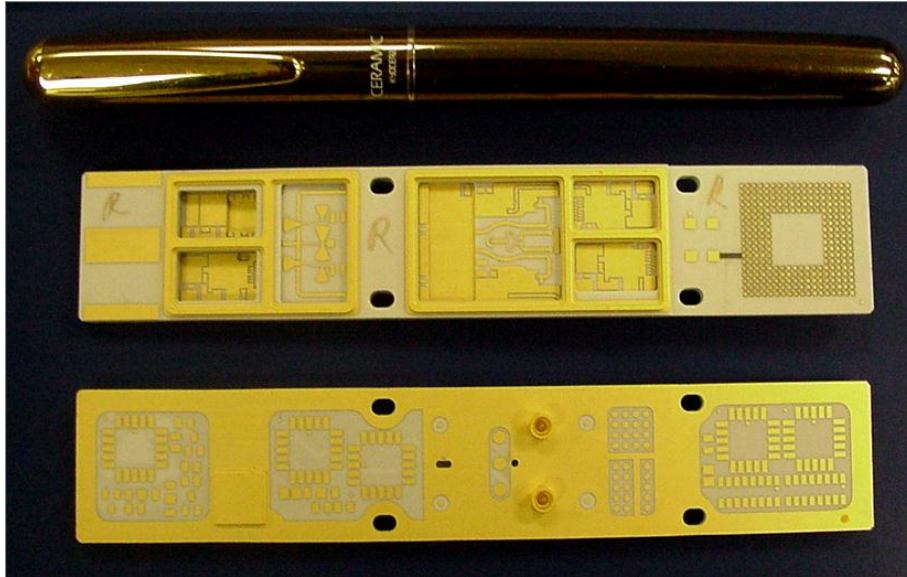
Fig. 1: T/R Module Package Courtesy of EADS Astrium [1]
