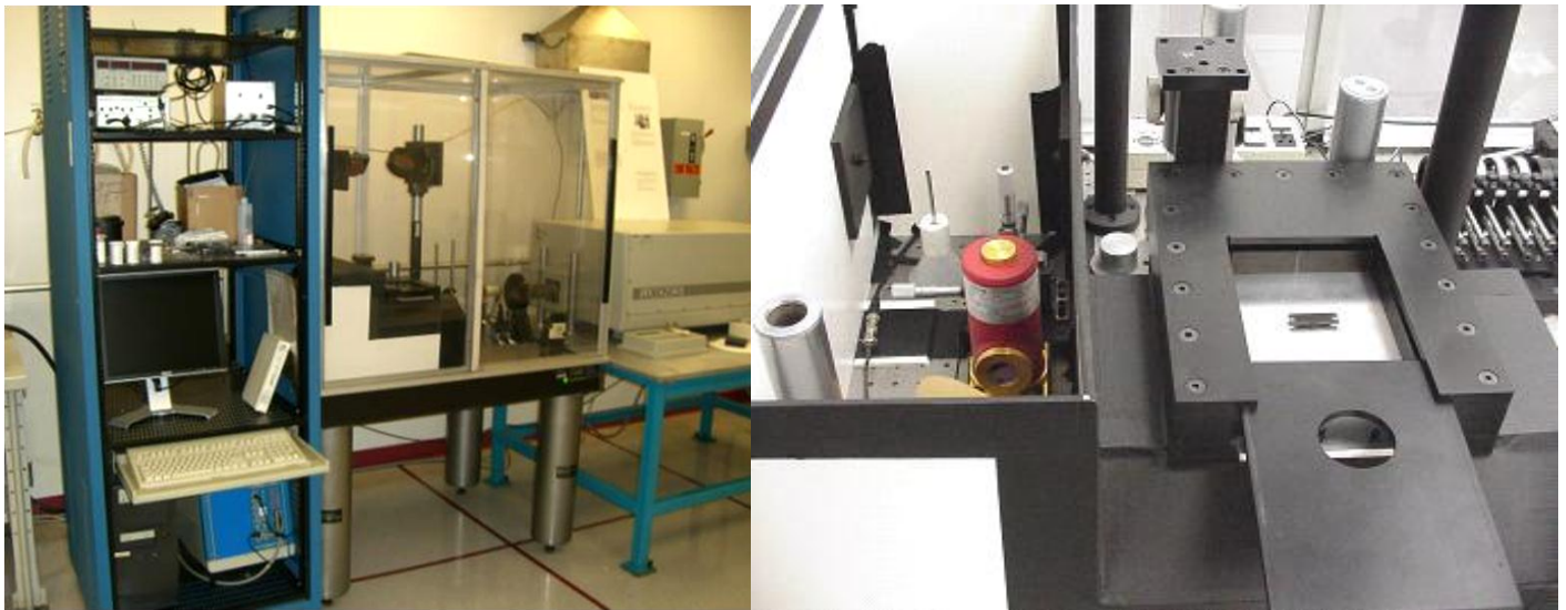
Fig. 5: Custom Laser Flash Experiment Setup used in Thermal Diffusivity Measurements.
